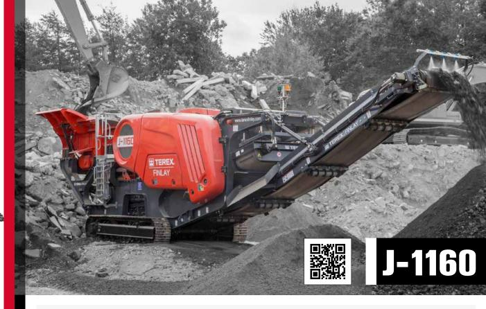
The Terex Finlay J-1160 is a compact and aggressive tracked mobile primary jaw crusher. Incorporating the Terex Jaques JW40 jaw crusher a heavy duty VGF feeder and an integrated prescreen system the Terex Finlay J-1160 gives optimum production in quarrying, mining, demolition and recycling applications.
