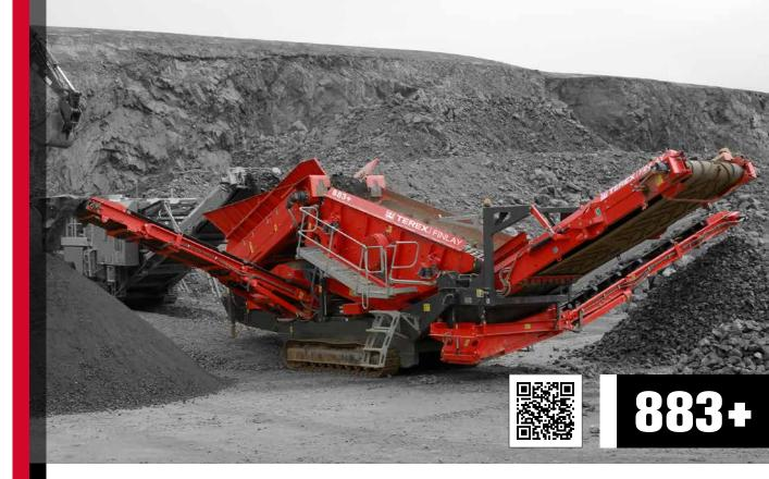
The high performance Terex Finlay 883+ is designed to work after a primary crusher or on it's own as a frontline tracked mobile screening machine. Applications include quarrying, mining construction and demolition debris, topsoil, recycling, sand, gravel, coal and aggregates. The plant has the capacity to process at a rate of up to 500 tonnes per hour and can be fed either by a tracked mobile crusher or an excavator.
