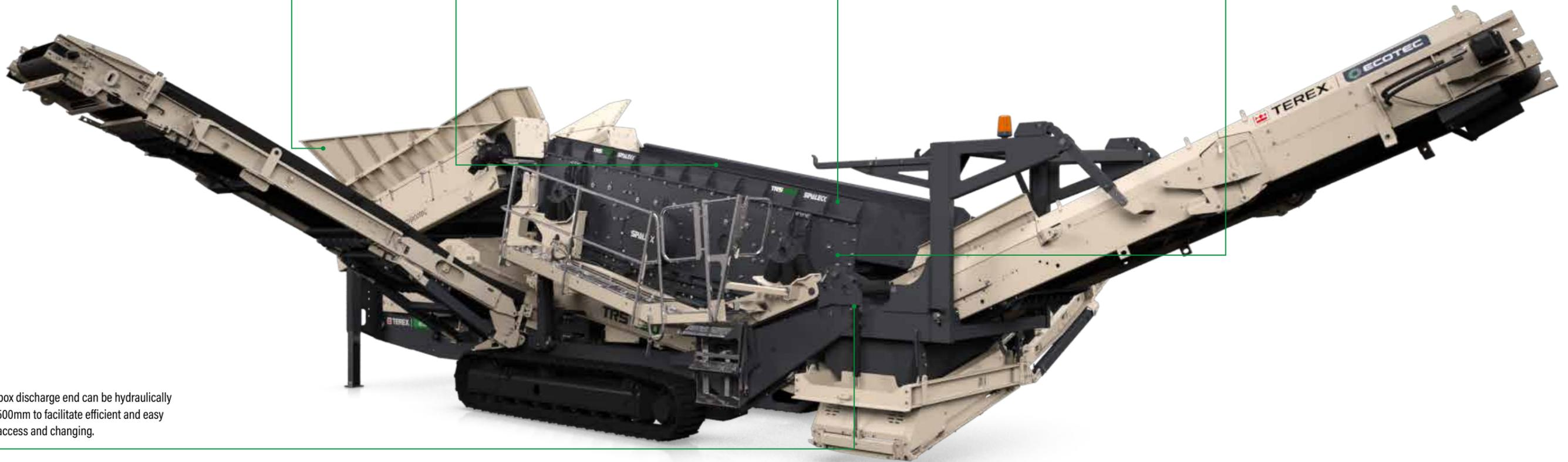
Screenbox discharge end can be hydraulically raised 500mm to facilitate efficient and easy media access and changing.
