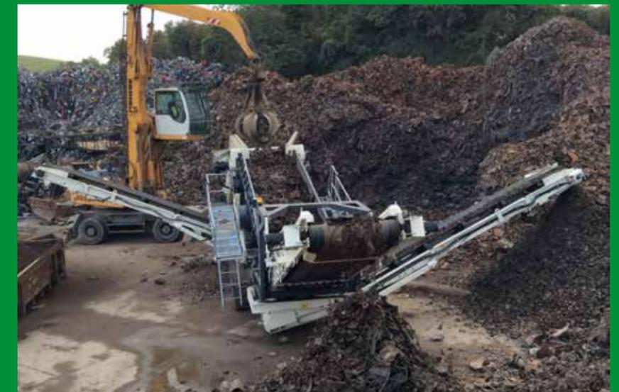
Terex® Ecotec's tracked heavy duty screen can be operated in a wide range of primary and secondary screening applications. The TRS 550 Recycling Screen features a two-deck German-designed recycling waste screen with Flip-Flow-Screen technology. This high-performance waste screen is combined with advanced technology on the bottom deck to elevate the TRS 550 into a class of its own.
