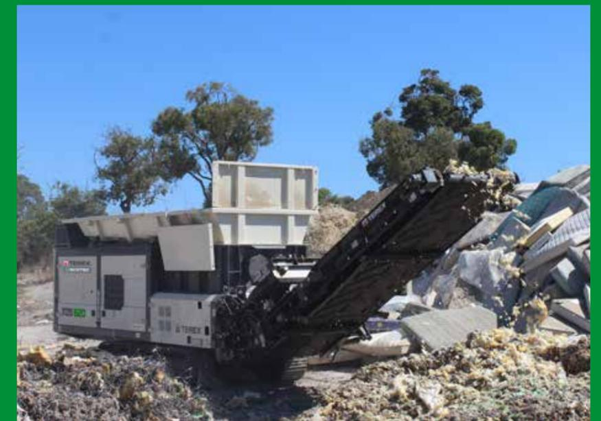
Key features include the hydrostatic drive offering better protection against contamination and allowing for bi-directional shredding. The double shaft shredder has 2m long shafts with a fully welded tooth configuration, impressive throughput and excellent reduction.
