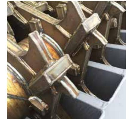
Shaft cutting elements are a fully welded structure with hard-faced edges giving ultimate strength in difficult applications
